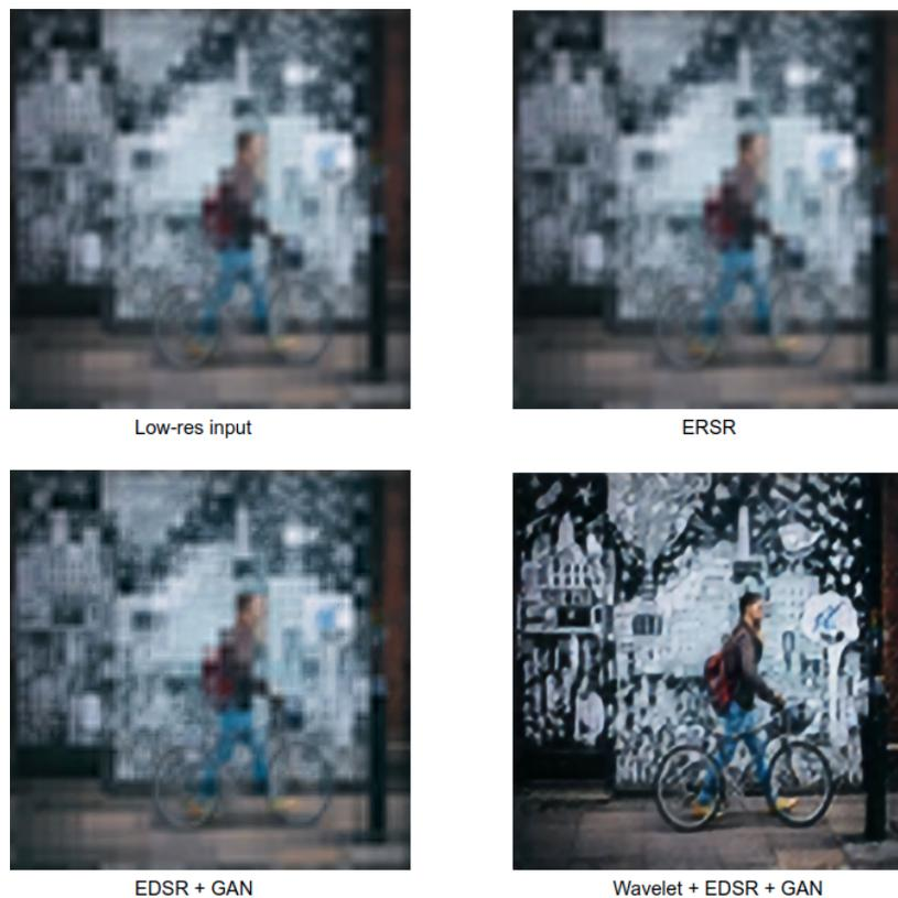
Fig. 9: Comparison between LR vs Wavelet processed-LR
